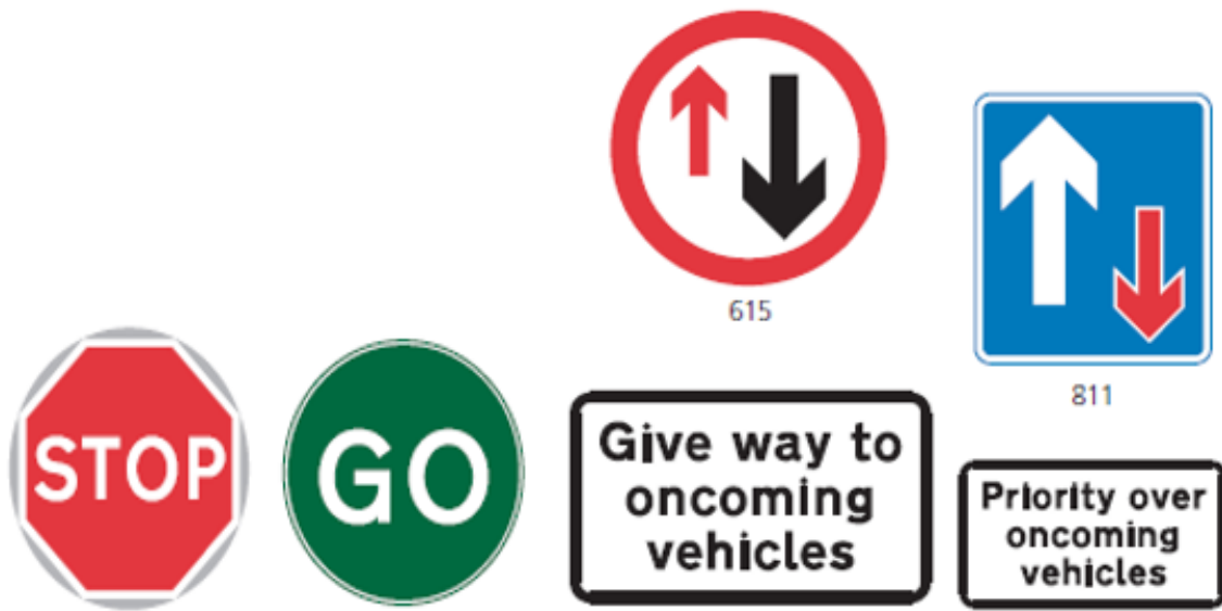
Figure 1.5: Manually operated stop/go signs and priority signs
